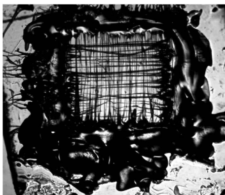
Fig. 6. Optical image of double layered scaffold with adhesives applied to the ends.
